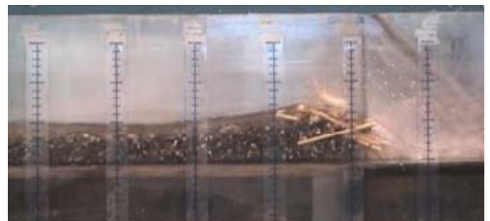
Figure 9. Flow situation 10 seconds after the arrival of the flow front at the open check dam.
